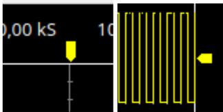
The trigger level (voltage) can be selected by dragging the small colored (e.g. yellow) arrow to the right of the recording window. The trigger position on the screen can be selected by dragging the colored (e.g. yellow) arrow at the top of the window.
