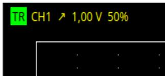
Trigger status (TR = triggered, TR = not triggered), source, slope, level and position are displayed in the upper left corner of the trace window.
