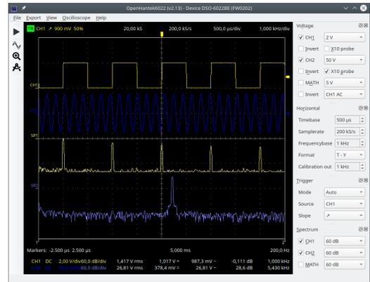
The digital storage scope Hantek6022BE (as well as the similar Hantek 6022BL) measures two voltage channels CH1 (yellow) and CH2 (blue).
