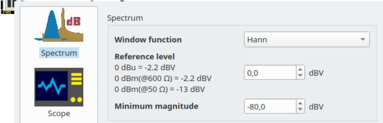
Typical window functions are Hann (raised cosine), Gauss or Flat top. The first window has the best frequency selectivity (narrowest bandwidth) while the last window allows accurate amplitude measurements. Gauss is in between.
