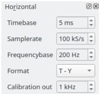
The displayed time range of the trace can be selected by Timebase between 10ns/div and 100 ms/div in 1/2/5 steps. The display's width is 10 div, marked with vertical dotted lines on the screen.
