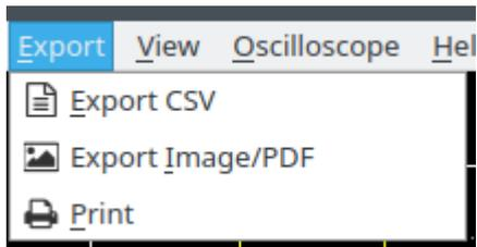
The Export CSV function allows to store the measured samples and the resulting spectral values as a \*.csv file (comma separated values).
