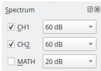
The program calculates the voltage spectrum of the three channels using the discrete FFT and displays the results if enabled. The displayed values are shown as dBV where 0 dBV equals 1 V rms.
